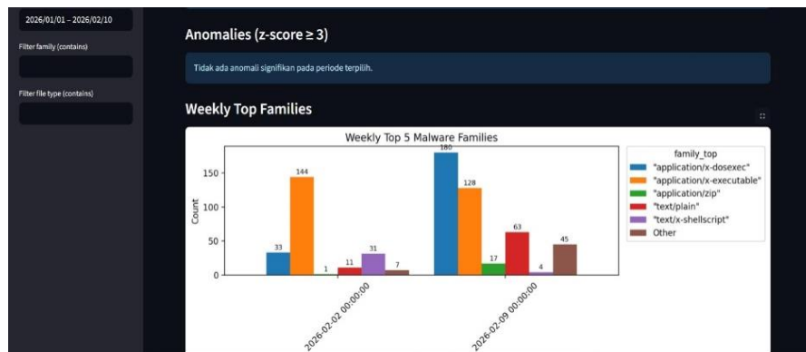
Figure 5. Malware Grouping Panel Based on malware activity and anomaly detection
