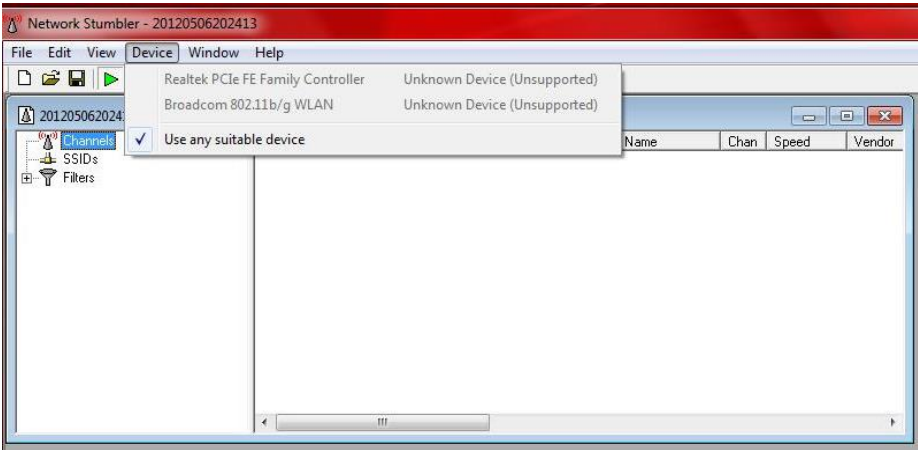
Figure 2. Network adapter device configuration in Netslumber software
